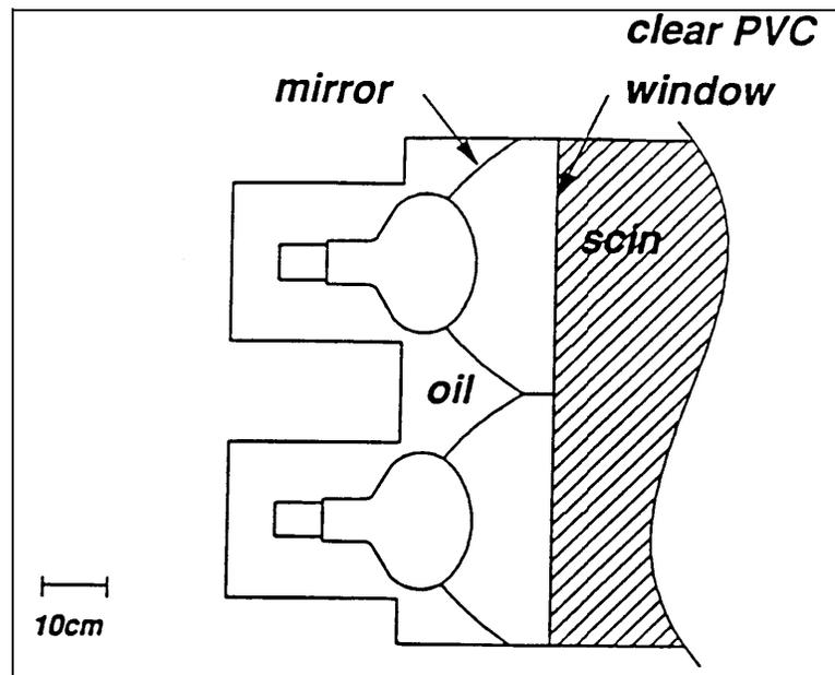
Figure 6: One end of a Horizontal Scintillator Box.
