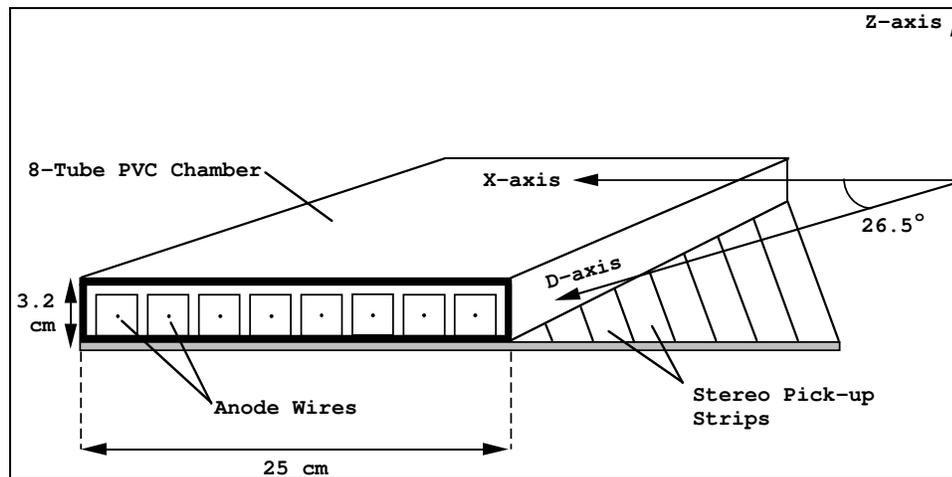
**Figure 5:** Schematic of a MACRO Streamer Tube Chamber.
