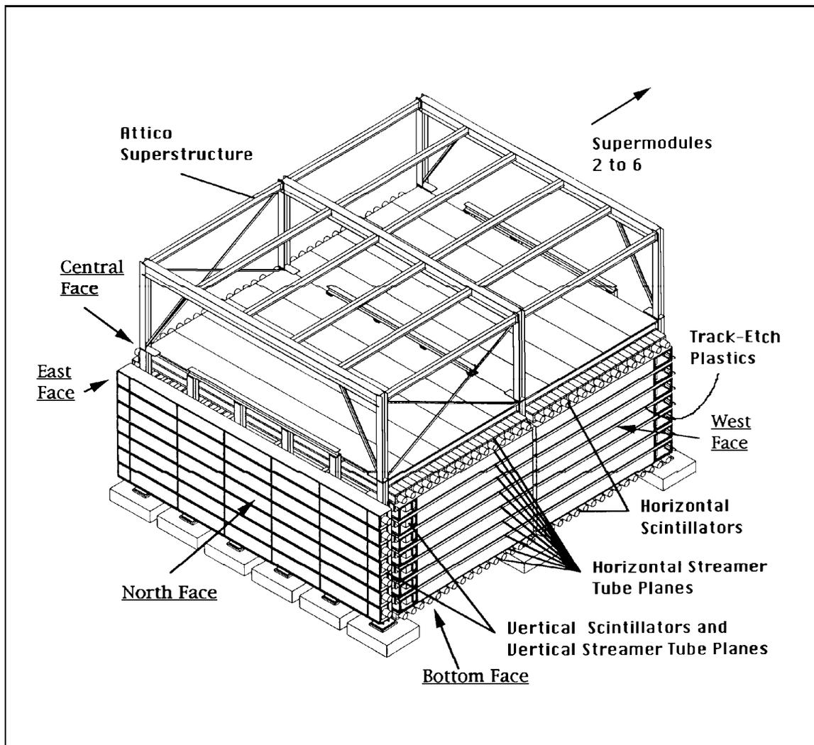
**Figure 3:** The first Supermodule of MACRO. Note the two modules of streamer tubes. The attico superstructure is also now laden with scintillator and streamer tube planes.
